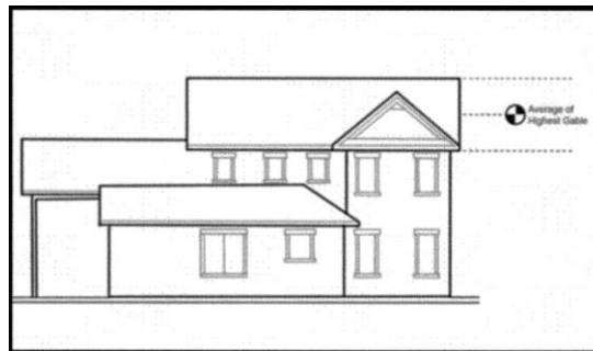
Gabled Roof(2 or More Gables) (Measured to the Average of the Highest Gable)
